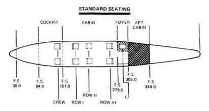
Okay, maybe this will help. In this diagram, notice that the various bulkheads in the airplane have F.S. numbers, and within each compartment, the seats will also have a F.S. number based on where it's actually bolted to the airplane. They're not shown on this diagram because the seats will be in slightly different places from airplane to airplane.
