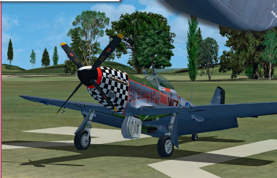
With the engine off, the pressure in the virtual hydraulic system 'bleeds down', and, as a result, the hydraulically controlled flaps and inner landing gear doors drop down realistically
